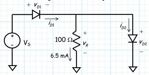
The diodes are identical, with n = 1 and  $I_s = 10^{-14}$  A.
